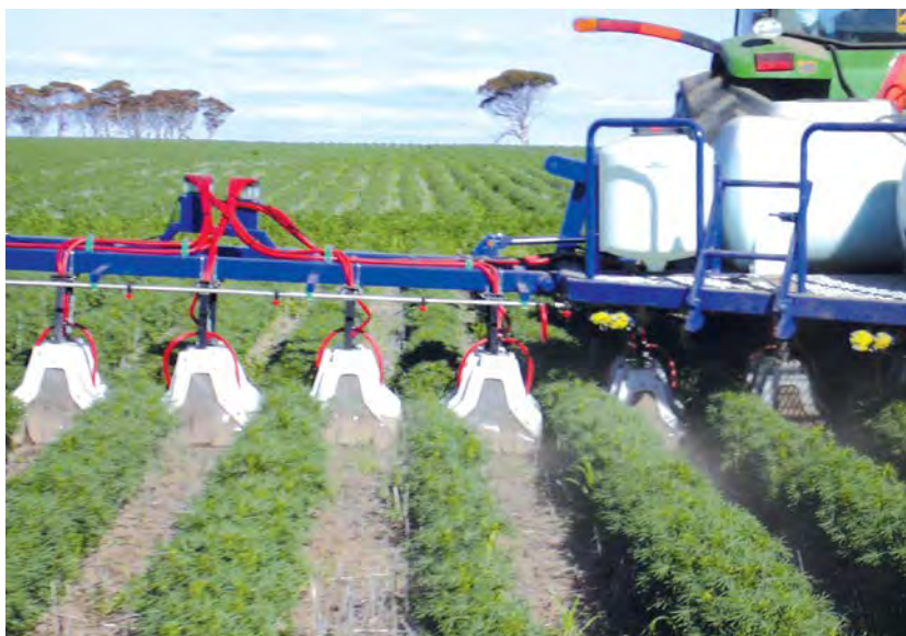
Shields being used to make lupins 'Roundup' Ready', by spraying glyphosate in between the rows.
