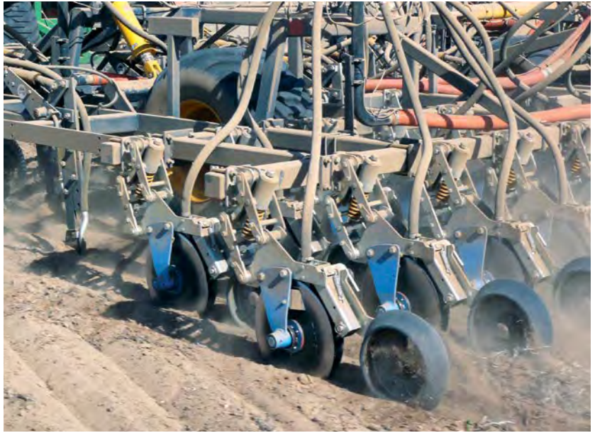
Primary Nichols seeder capable of deep sub-soil tillage while 'no-tilling'.
