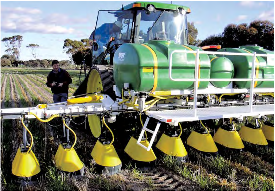
A TPos shielded sprayer for inter-row spraying of herbicide resistant weeds.
