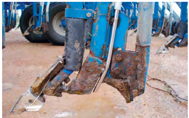
Liquid fertiliser is injected behind the knife opener.
