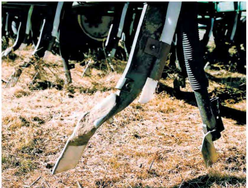
The original Agmore closer tool. It is now made with plastic and is quite popular.
