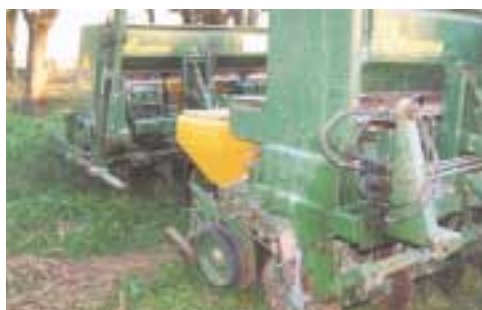
Roberto Perretti's seeder units that can be pulled behind each other to sow cool season grasses (wheat) or put alongside each other to sow warm season crops on wider row spacings.
