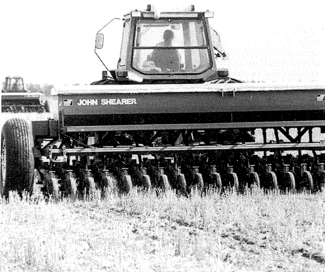
John Shearer Combine fitted with Walker Double Discs
